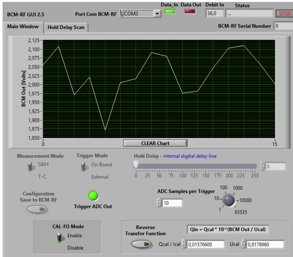
When CAL-FO Mode is enabled, the BCM-RF-E operates in Sample & Hold mode and uses the On-board trigger. The BCM-RF system GUI thus automatically triggers after a pulse occurred at the Turbo-ICT input.
