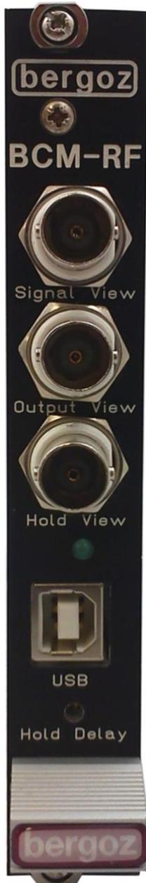
**Signal View:** BNC connector, waveform to be read by oscilloscope (50  $\Omega$  or 1 M $\Omega$ )
